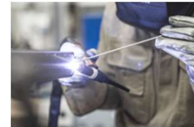
TIG welding on a component
